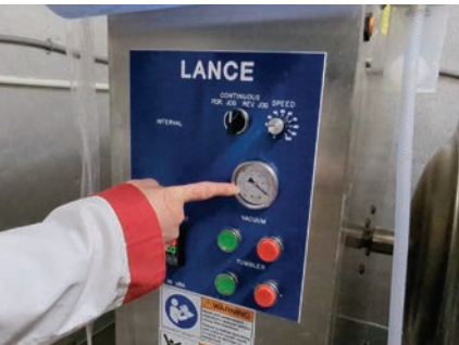
13. Run vacuum pump until 15 inches of vacuum (or desired level) is drawn.
