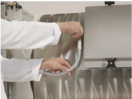
14. Shut off the valve on the drum.
