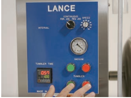
21. Press tumbler start button, The drum will now rotate until the tumbler timer runs down to zero.
