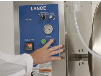
16. Turn off the vacuum pump.
