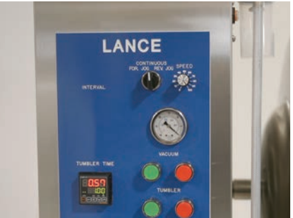
19. Set the mode switch to continuous.
