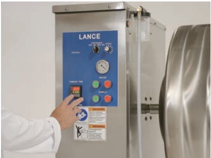
17. Set the tumbler timer to the desired time.
