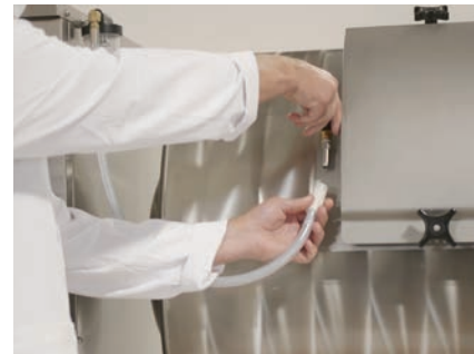
12. Push vacuum hose onto drum fitting.
