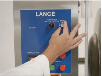
18. Set variable speed knob to the desired speed.
