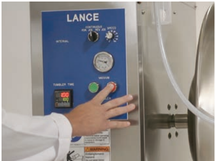
16. Turn off the vacuum pump.
